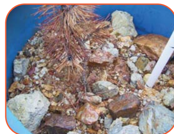
Growth trials within one of the Gilt Edge Mine drums containing a waste rock and Acid B™ reagent mixture.
