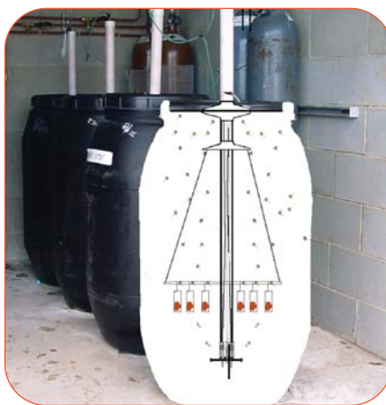
Figure 1 - Schematic cross-section of the anoxic and anoxic-reducing drums.
